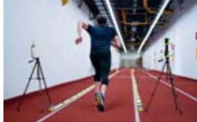
A 30-meter optical measurement system consisting of a transmitting and receiving bars detects any interruptions in communication between the bars and calculates their duration.
