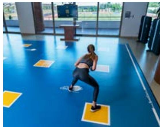
The SpeedCourt is a multifunctional training and measurement system for speed and agility, coordination, visual and cognitive perception and end stage rehabilitation. On a sports floor field of 50m², 12 sensor fields are embedded, connected and steered by highly sophisticated software. Variations of fundamental, motion, explosiveness and reactive speed, acceleration and agility, power, and injury prevention can be created by the coach and be visualized on a large screen for the athlete.
